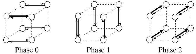
Figure 10: Recursive doubling algorithm for eight processes
