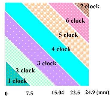
Figure 5: Illustration of how far each clock can travel to cross the global interconnects. Assume a die of 24.9mm x 24.9mm in the 0.07 $\mu$ m technology with a 5 GHz clock as predicted in NTRS'97 [2]. Optimal buffer insertion and wire-sizing are performed using the TRIO package [3] with the driver, buffer, and receiver sizes being 100x the minimum size inverter. Device and interconnect parameters are based on those presented in [4].
