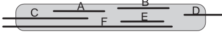
Figure 9: Illustration of Onodes/Rnodes. The shadow area is a power rail. All segments inside are Onodes. A, B and D have no parent nodes in this power rail. Thus A, B and D are URnodes. F and E have no child nodes in this power rail. They are DRnodes. A node can be both URnode and DRnode, like D.
