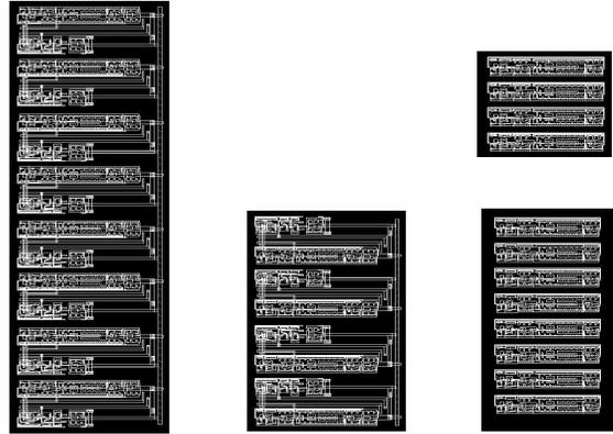
Figure 11: Layout of the CRT drivers
