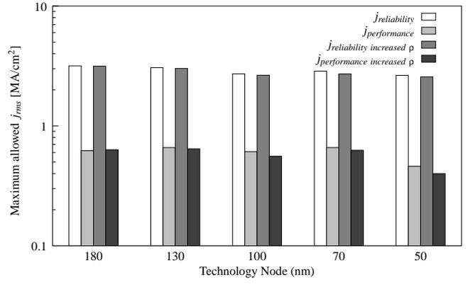
Figure 10: Comparison of  $j_{rms}$  values obtained from reliability and electrical performance considerations for top layer metal for various ITRS technology nodes with and without taking into account increased resistivity due to surface scattering and barrier materials.
