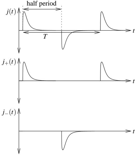
Figure 3: A bipolar pulsed waveform illustrating various current definitions.
