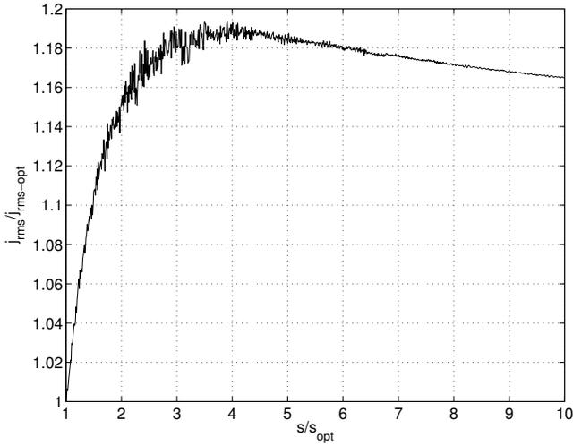
Figure 12:  $j_{rms}$  as a function buffer size for an interconnect length of  $l_{opt}$  for the 100 nm technology node.
