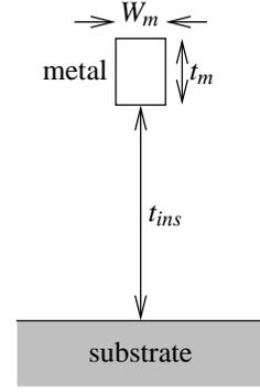
Figure 1: Cross-section of a metal interconnect over Silicon substrate.
