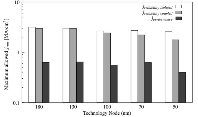
Figure 11: Maximum allowed  $j_{rms}$  for top layer metal of ITRS technologies for symmetric bipolar currents with and without thermal coupling from neighbouring lines. Also shown is the  $j_{rms}$  from performance considerations.
