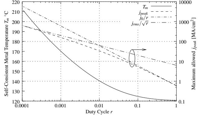
Figure 2: Self-consistent solutions of  $T_m$  and  $j_{peak}$  for metal 6 of 180 nm technology node with  $j_0 = 0.6$  MA/cm<sup>2</sup>,  $\rho_m(T_m) = 2.7 \times 10^{-6} [1 + 6.8 \times 10^{-3}/K \times (T_m - T_{ref})]$   $\Omega\text{-cm}$ ,  $T_{ref} = 120^\circ\text{C}$  and  $Q = 0.5$  eV. The two dotted lines indicate  $j_{peak}$  based on (a)  $j_{peak} = \frac{j_0}{r}$  and (b)  $j_{peak} = \frac{j_{rms}}{\sqrt{r}}$ .
