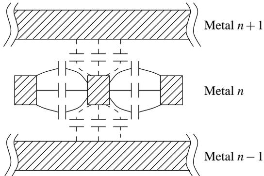
Figure 8: Typical metal interconnect structure.
