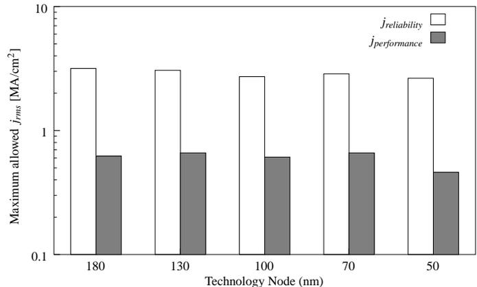
Figure 9: Comparison of  $j_{rms}$  values obtained from reliability and electrical performance considerations for top layer metal for various ITRS technology nodes.
