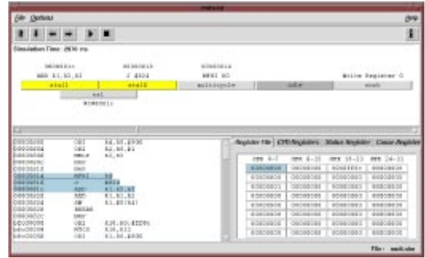
Figure 5. Snapshot of the graphical validation tool: The pipeline displayed executes an instruction in the write-back stage, and the memory stage is idle because the execute stage operates on a multicycle operation. This operation stalls the instruction decode and address translation phases, while the instruction fetch is allowed to complete (the stage is in state CAL, i.e., cache access load).
