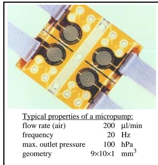
**Figure 2. Modul of four micropumps**
