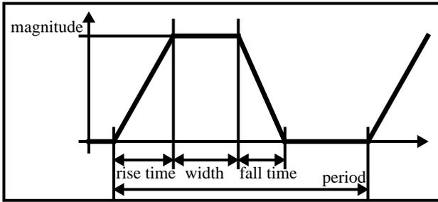
**Figure 4. Power supply of the micropump**
