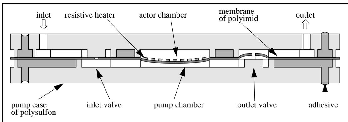
Figure 3. Schematic view of the micropump
