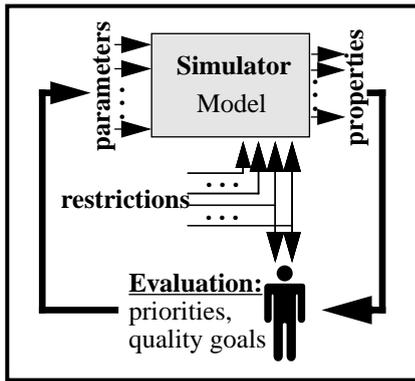
**Figure 1a. Conventional Design Process**
