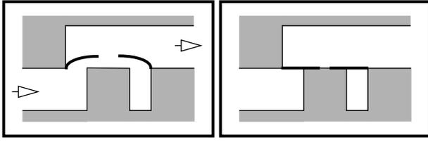
Figure 6a. Opened valve Figure 6b. Closed valve
