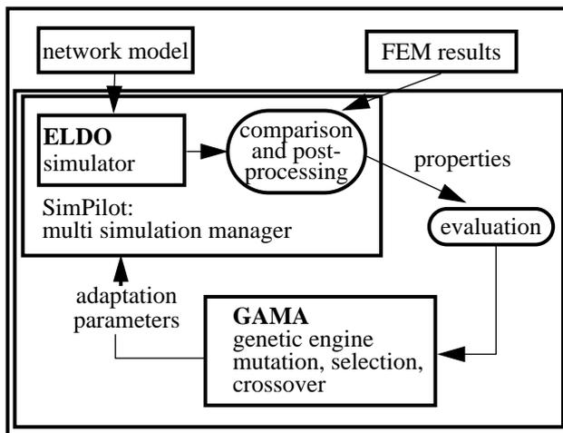
Figure 7. Scheme of the model adaptation process
