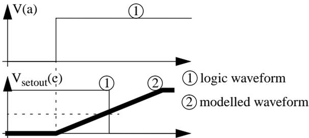
**Figure 8: Ramp construction to make peak voltage estimation possible for [7]**
