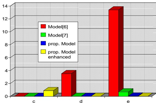
**Figure 12: Relative amount of cases which result in no transition for circuit-level simulation and a hazard for the gate-level model in %**
