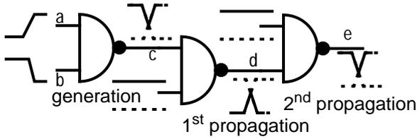
**Figure 7: Benchmark circuit for evaluation of glitch model**
