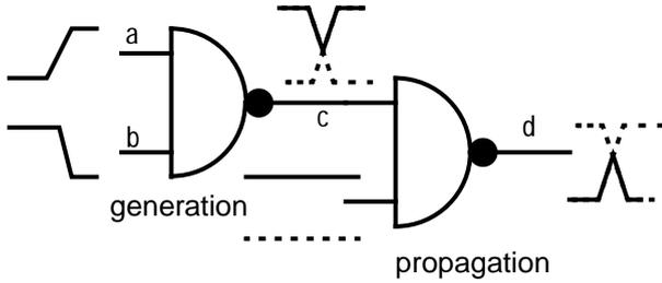
**Figure 3: Representation of glitches by linear approximated ramps**
