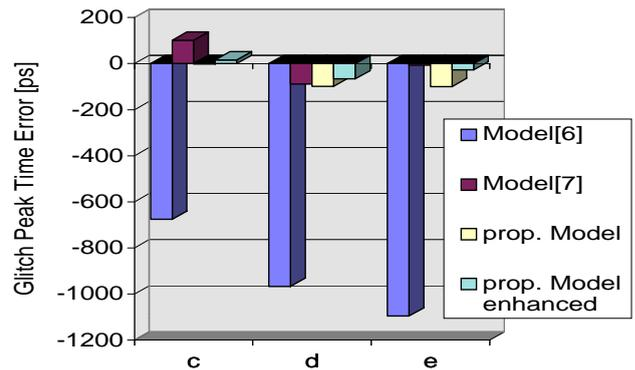
**Figure 11: Mean value of glitch peak time error**
