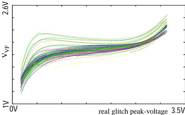
**Figure 6:  $V_{VF}$  of a NAND2-gate for different circuit configurations**
