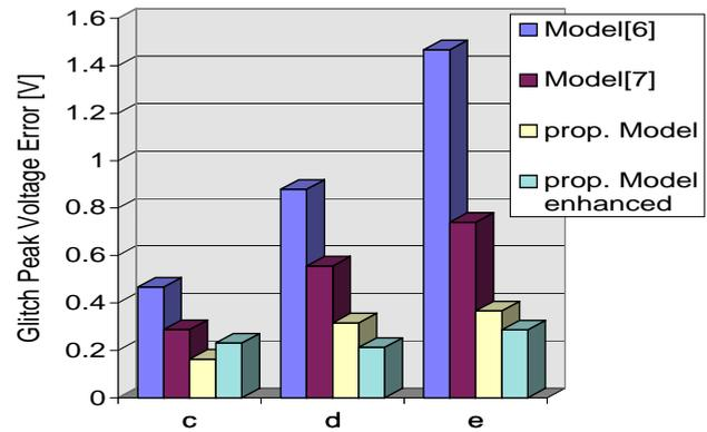
**Figure 10: Standard deviation of glitch peak voltage error**
