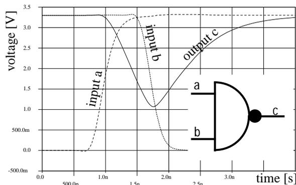
Figure 1: Example for a glitch at a NAND2-gate
