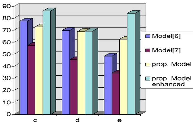
**Figure 13: Relative amount of simulated glitches on circuit-level which are detected by the gate-level model in %**
