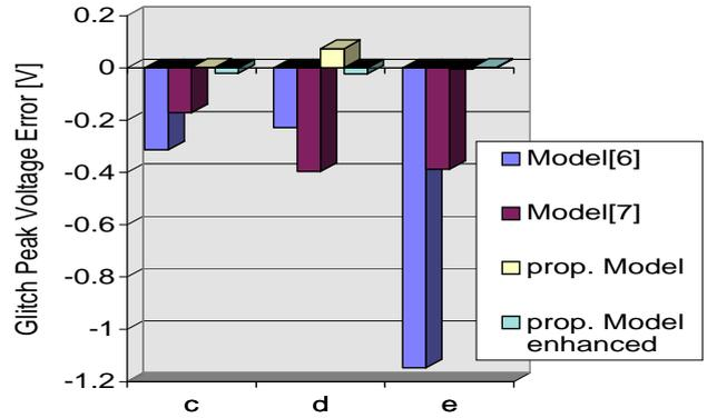
**Figure 9: Mean value of glitch peak voltage error**
