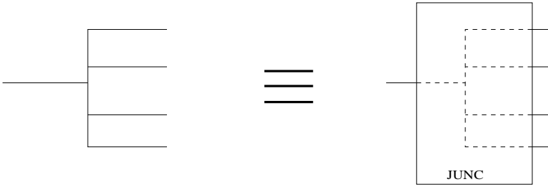
Figure 5: A junction can be treated as a multi-output gate.
