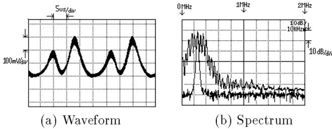
Fig. 6. Noises from a HF lamp
