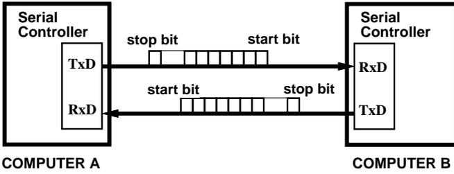
Fig. 1. Serial communication system
