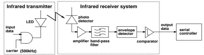
Fig. 8. ASK receiver using envelope detector
