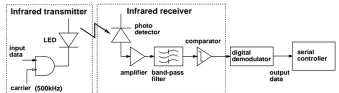
Fig. 9. ASK receiver using digital demodulator
