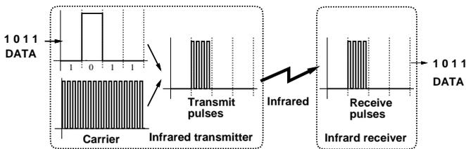
Fig. 3. Amplitude Shift Keying
