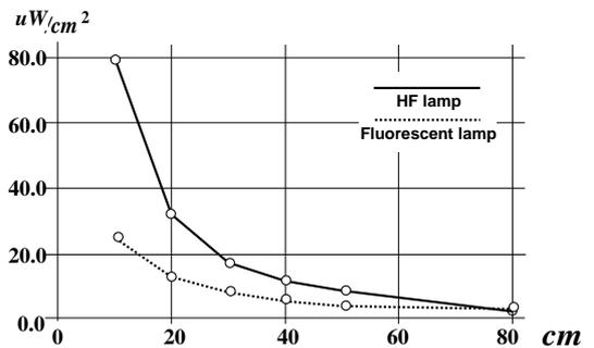
Fig. 5. Intensity of optical noise from lamps
