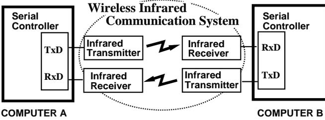
Fig. 2. Serial communication system by wireless infrared communication
