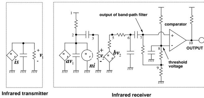
Fig. 10. Model of infrared communication
