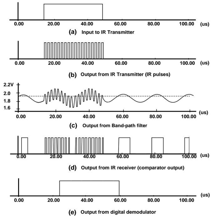
Fig. 11. Outputs of infrared receiver with modeled noises
