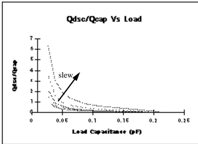
Figure 1: Ratio of dynamic short-circuit charge to capacitive charge as a function of load capacitance and input slew. For large slew and small capacitance the dynamic short-circuit charge exceeds the capacitive charge.
