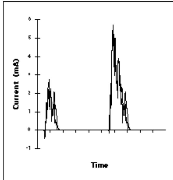
Figure 10: Instantaneous current waveforms from Lsim Power Analyst and Eldo for a 4-bit adder circuit.
