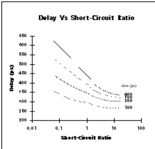
Figure 9: Variation of delay with short-circuit ratio for different input slew and fixed load capacitance.
