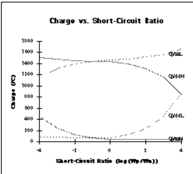
Figure 4: Total and short-circuit charge variation with short-circuit ratio.
