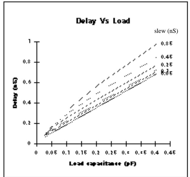
Figure 8: Delay variation with load capacitance and input slew.
