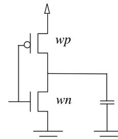
Figure 2: Inverter for characterizing charge and current.
