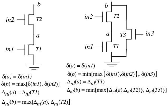
Figure 5: Propagation of input slew across series-parallel components.
