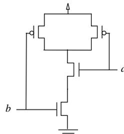
Figure 7: Nand gate example shown in Table 1.
