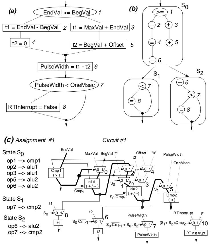
Figure 3: The UAV example for illustrating statically unsensitizable paths due to implicit sharing across states.
