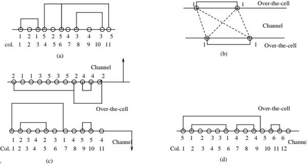
Figure 2: (a) Planar routing over the cell; (b) possible net segment connecting two hyperterminals; (c) A valid solution for TFPR (height is 3); (d) a valid solution to OFPR (height is 2).
