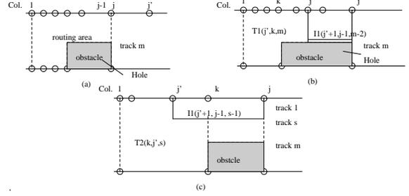
Figure 4: (a) An instance with  $j'$  out of routing region; (b) An instance with  $k \leq j' < j$ ; (c) An instance with  $1 \leq j' < k$ .
