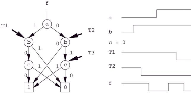
Figure 4: BDD implementation with ordering  $a < b < c$ .
