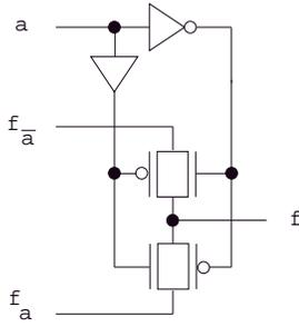
Figure 2: A transistor-level implementation of a hazard-free multiplexor.
