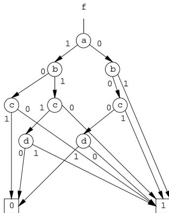
Figure 7: Dynamic hazard free BDD implementation with ordering  $a < b < c < d$ .
