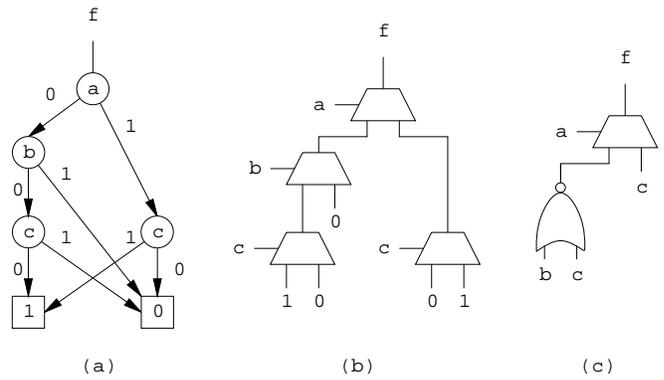
Figure 1: (a) A BDD. (b) The derived multiplexor multilevel network. (c) Simplification of multiplexors by constant propagation.
