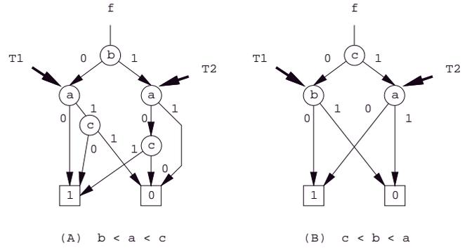
Figure 5: BDD implementation with orderings (a)  $b < a < c$  and (b)  $c < b < a$ .
