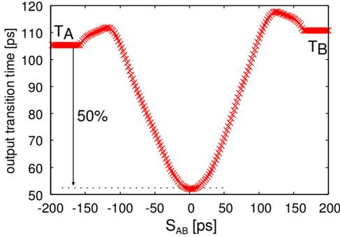
Fig. 6. Example of the output transition time of rising output transition
