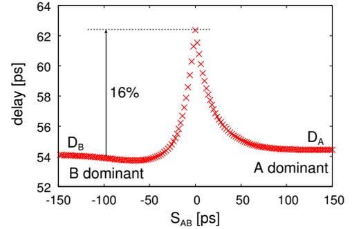
Fig. 4. Example of the gate delay of falling output transition
