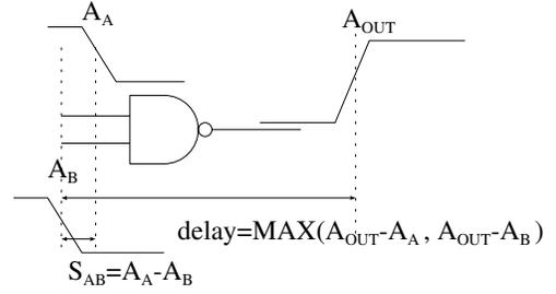
Fig. 3. Gate delay of rising output transition
