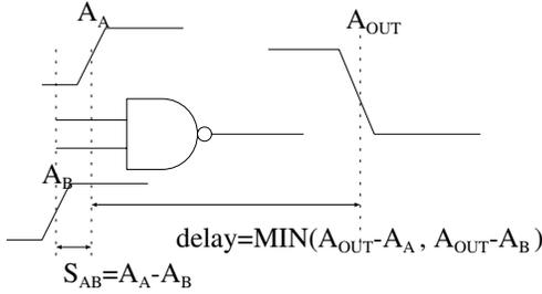
Fig. 2. Gate delay of falling output transition
