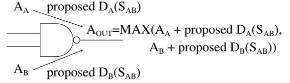
Fig. 7. Proposed gate delay model for MIS
