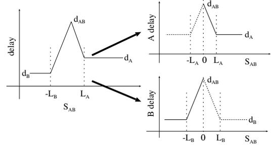
Fig. 8. Proposed calculation method of gate delay
