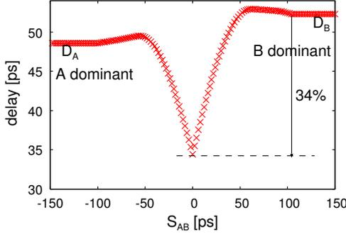
Fig. 5. Example of the gate delay of rising output transition
