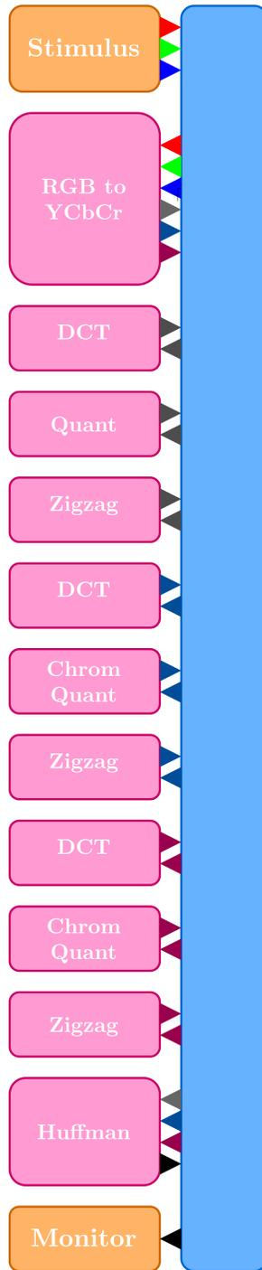
Figure 18: The mapping of the JPEG encoder application to the CMA.
