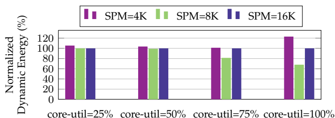
Fig. 18: Dynamic energy in memory subsystem and network: CNGLSA normalized to CNA.
