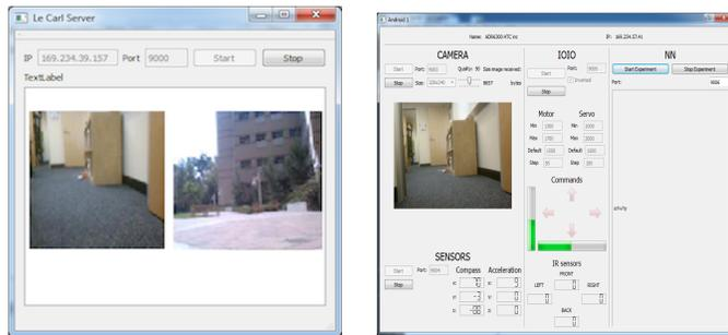
**Figure 7.** Server program running on a computer. Left - multiple phones/robots can connect to the server and stream data such as video feed. Right - Interface for one robot. Using this window, users can start/stop streaming the video, sensory information coming from the compass, accelerometer, and IR sensors connected to the IOIO. They can also control the robot using the keyboard or allow the robot to run in autonomous mode.
