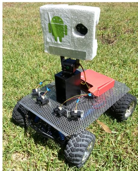
**Figure 3.** Android based robotic platform composed of IOIO, four infrared sensors, and a robotic head mounted onto a perforated steel base. The base is installed on the chassis of a R/C truck. The robotic head is composed of a rectangular tube, two servos for the pan and tilt unit, and a phone holder made of foam.
