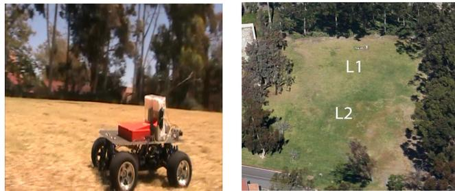
**Figure 10.** Left – Android based robotic platform with four infrared sensors and a protection case for the IOIO. Right - open grass field with both locations  $L_1$  and  $L_2$ , where the experiment was conducted.
