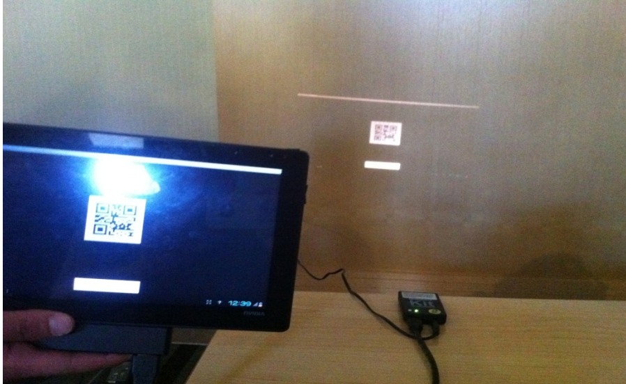
Figure 5.3: Pico Projector Displaying View from Tegra Tablet
