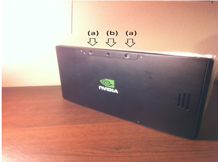
Figure 3.1: Camera (a) and Sensor (b) Locations on Tegra Board
