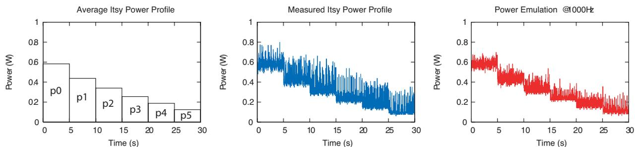
Figure 5: Comparison of Itsy power profile to load emulation waveform
