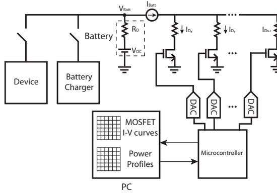
Figure 2: Power emulator circuit diagram
