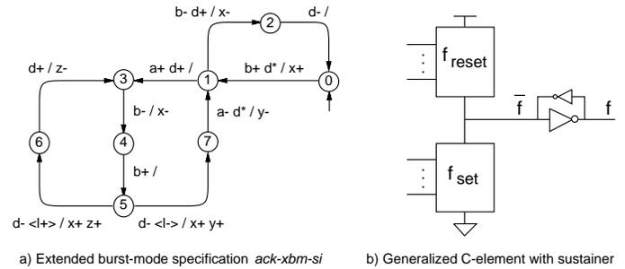
Figure 1. Extended burst-mode specification and gC implementation structure.
