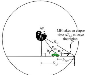
Figure 2: A MH is moving at a velocity  $v$  with a direction indicated by  $\theta_1$ .
