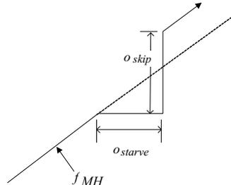
Figure 3: Illustration of hiccup factors:  $o_{starve}$  and  $o_{skip}$ .
