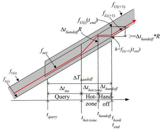
Figure 1: The seamless stream handoff process illustrated by the address constraints associated with two AP-MH connections.
